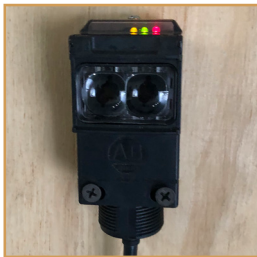
Photo-eye with 10-foot maximum range
