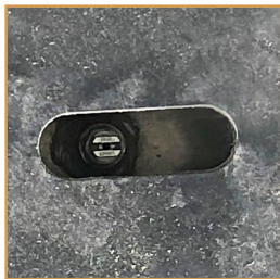
Twelve 15°, size 20 nozzles spaced 6-inches apart
