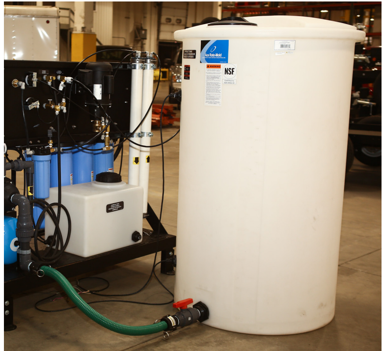
250-gallon holding tank
