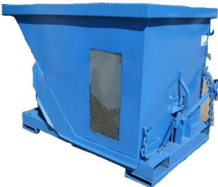
For solids handling, self-dumping dewatering hoppers from ¼ yard to 5 yards in size are available. Dewatering screens are stainless steel mesh behind stainless steel perf plate with ½” openings. The hopper is carbon steel with an option to come painted or galvanized.
